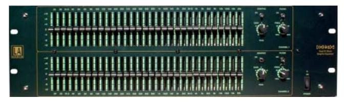
31 band pass filters based around precision minimum phase active RC networks deliver superior dynamic range and signal to noise performance. 45mm long throw faders provide maximum sensitivity and control of 12dB cut and boost at ISO centre frequencies from 20Hz to 20KHz.
